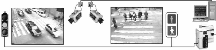
**Fig. 1.** In our prototype one camera focuses on the pedestrians and the other one on the vehicles. Images are then sent to the computer and as result a final working mode is sent to the automaton responsible for the traffic light switch.
