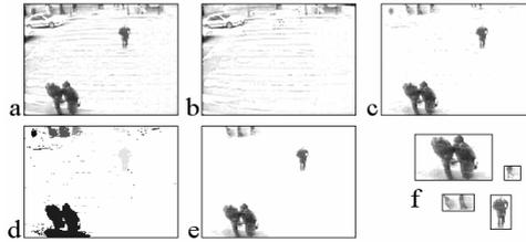
**Fig 3.** **a.** Source image taken at the pedestrian crossing. **b.** Background image computed with the mode of consecutive frames. **c.** Subtracted image with no background. **d.** Convex hull of every component labelled in a grey code. **e.** Final filtered image, without spurious components. **f.** Individual components to be tracked through the Kalman filter.
