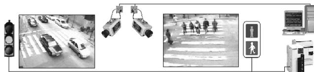
**Fig. 1.** General scheme of the prototype. Two cameras: one of them focussing on the pedestrians and the other one on the vehicles. Images are then sent to the computer and as result a final working mode is sent to the automaton responsible for the traffic light switch.
