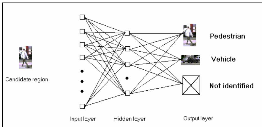
Figure 5.- Artificial Neural Network scheme.
