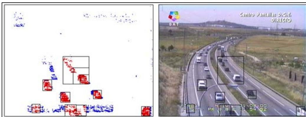
Figure 7. Detection of moving objects.
